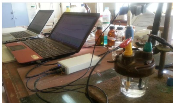
Figure 5. The apparatus used for cyclic Voltammetry
