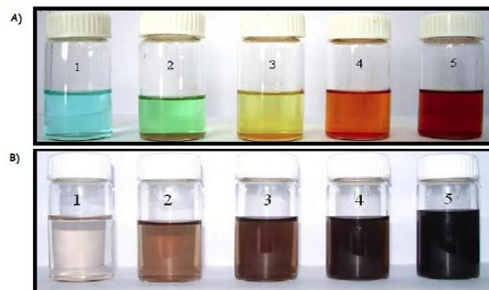
Figure 1. Change of colour during synthesis of copper nanoparticles in A) Water B) Glycol. Reprinted with the permission from copyright 2009 Nanoscale Res Lett
