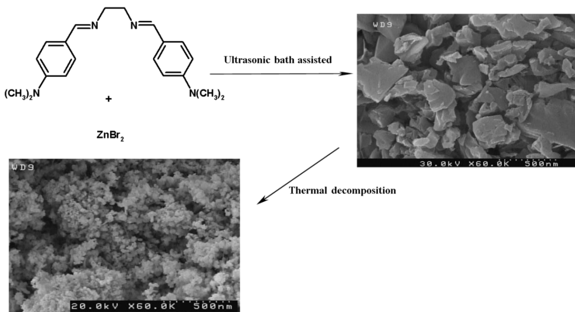
Scheme 1. Schematic for preparation of nano-size of zinc(II) Schiff base complex and ZnO nanoparticles
