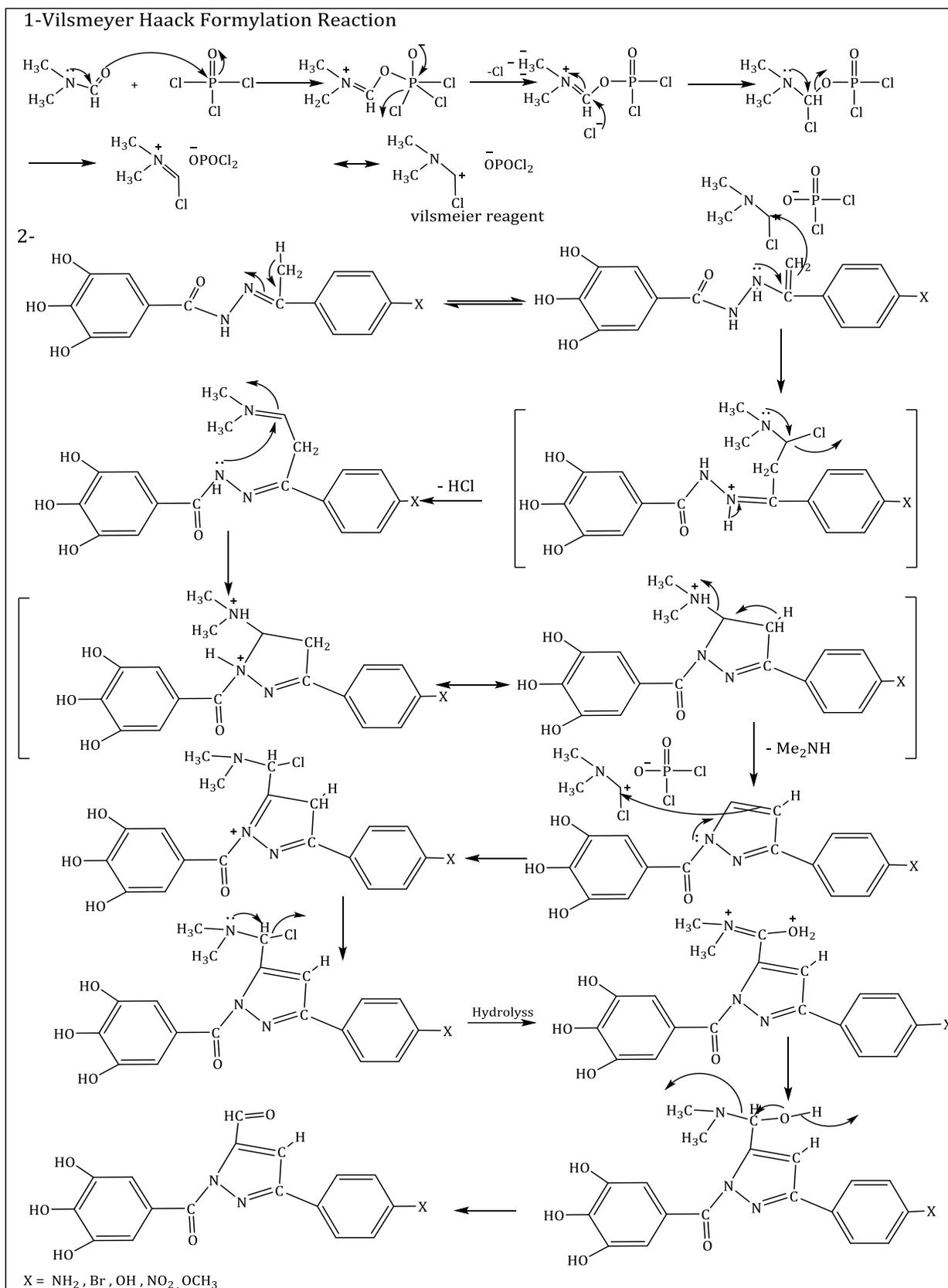
**Scheme 2:** The mechanism to obtain the newly synthesized 4-Formyl pyrazole derivatives
