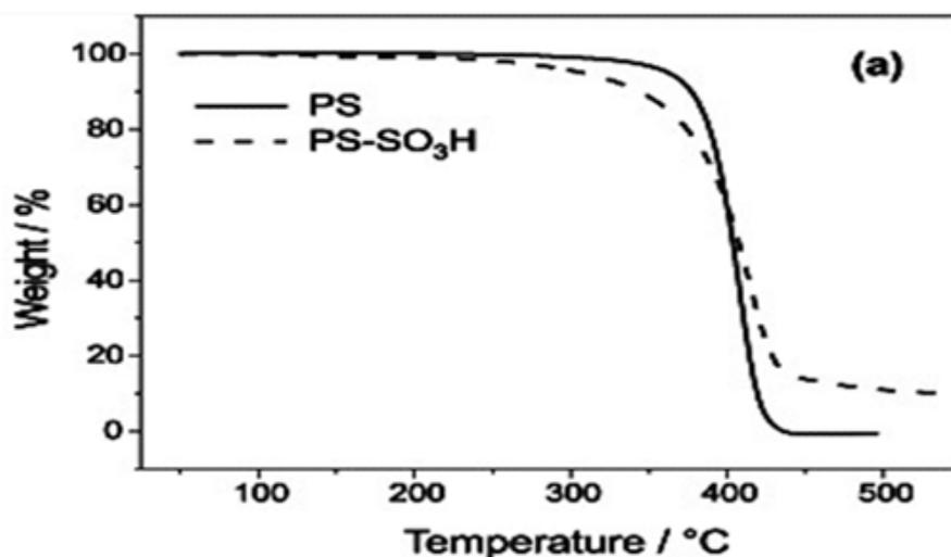
**Figure 2:** TGA thermogram of polystyrene and sulfonated polystyrene
