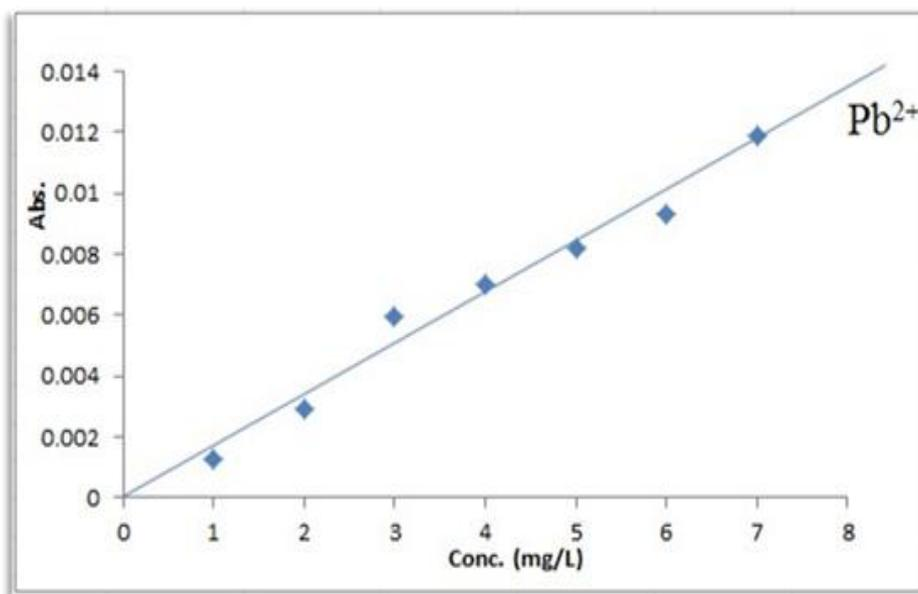
**Figure 6:** The calibration curve for Pb(II)
