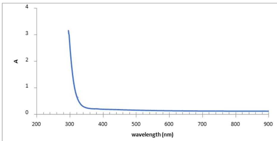
Figure 11: UV-Visible spectrum of SPS thin film
