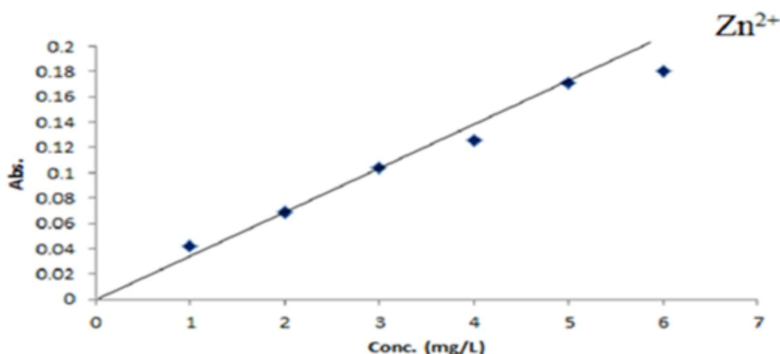
Figure 4: The calibration curve for Zn(II)
