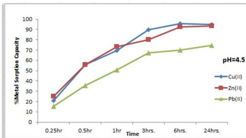
**Figure 8:** Percentage of metal sorption capacity at pH 4.5 by resin as a function of contact time
