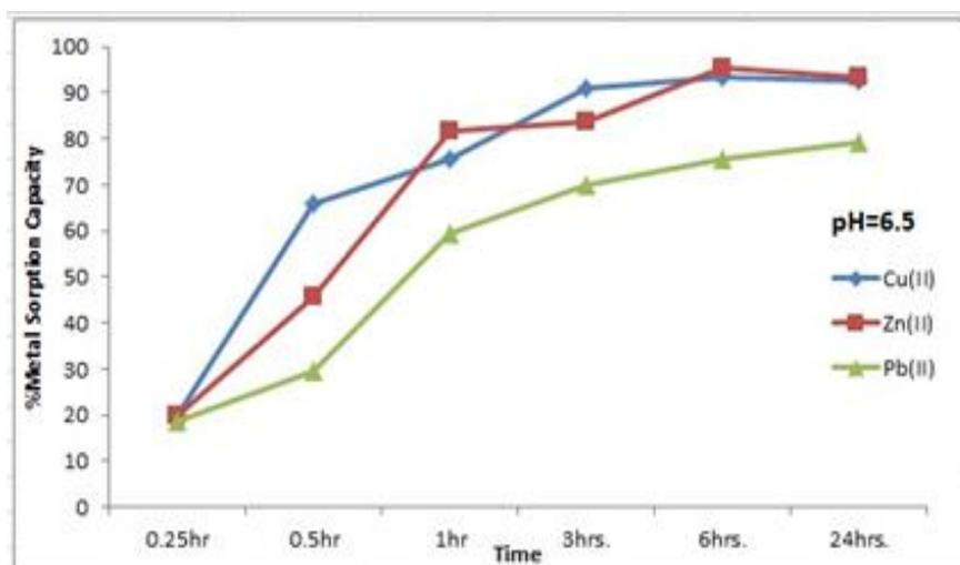
**Figure 9:** Percentage of metal sorption capacity at pH 6.5 by resin as a function of contact time
