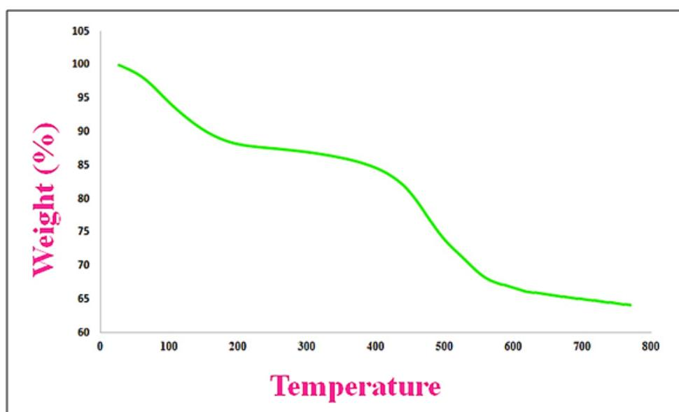
**Figure 2:** TGA curve of  $\text{Fe}_3\text{O}_4@\text{SiO}_2@\text{Mel-Rh-Cu}$
