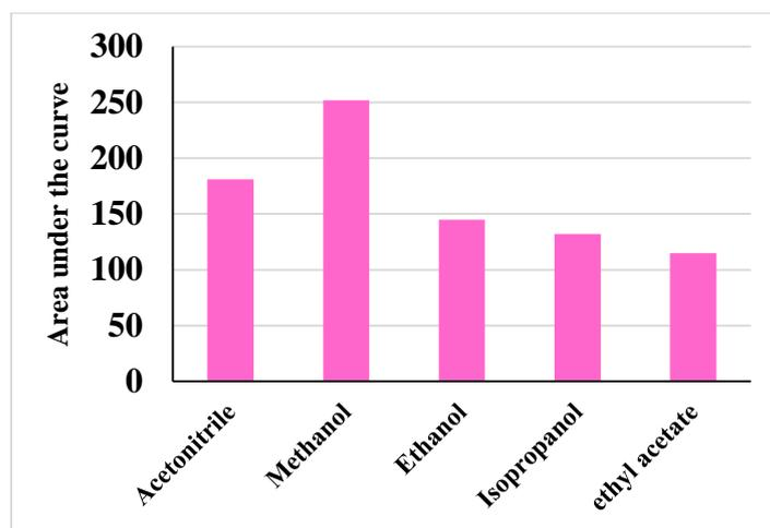
**Figure 8:** The effect of type of desorption solvent on magnetic solid phase microextraction process
