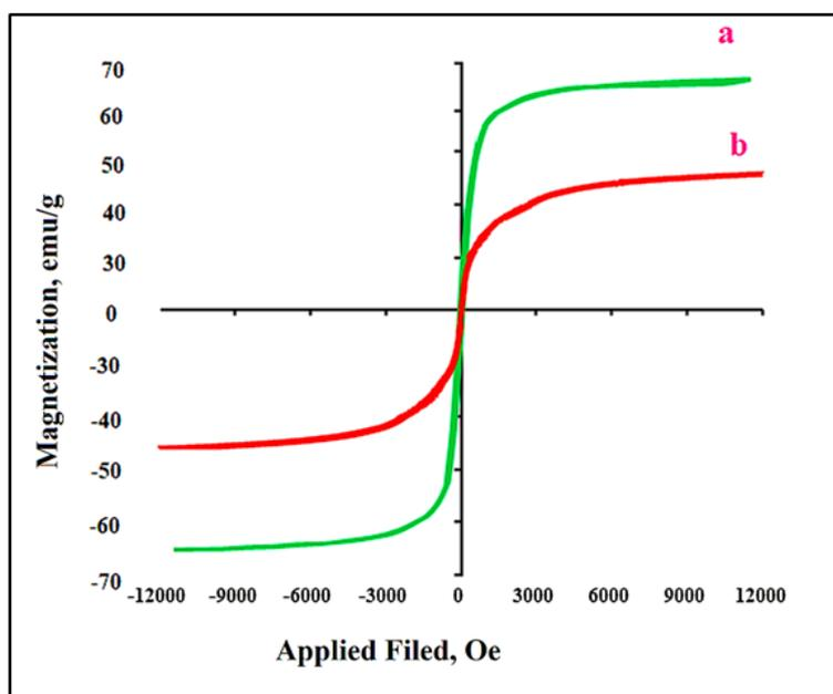
**Figure 7:** Magnetization curves of (a)  $\text{Fe}_3\text{O}_4$  and (b)  $\text{Fe}_3\text{O}_4@SiO_2@Mel-Rh-Cu$
