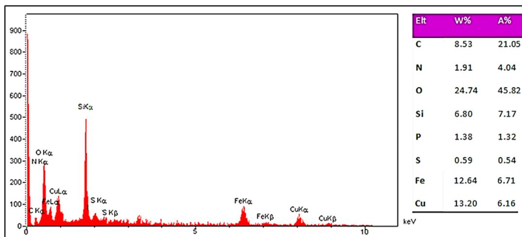
Figure 5: EDx pattern of Fe<sub>3</sub>O<sub>4</sub>@SiO<sub>2</sub>@Mel-Rh-Cu
