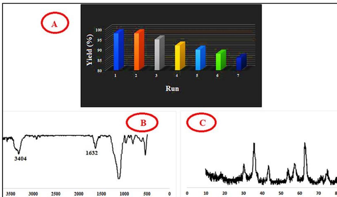
**Figure 9:** (A) Catalyst reusability diagram of the model reaction, (B) IR spectra of  $\text{Fe}_3\text{O}_4@\text{SiO}_2@\text{Mel-Rh-Cu}$  reused after seven cycles, and (C) XRD patterns of  $\text{Fe}_3\text{O}_4@\text{SiO}_2@\text{Mel-Rh-Cu}$  reused after eleven cycles
