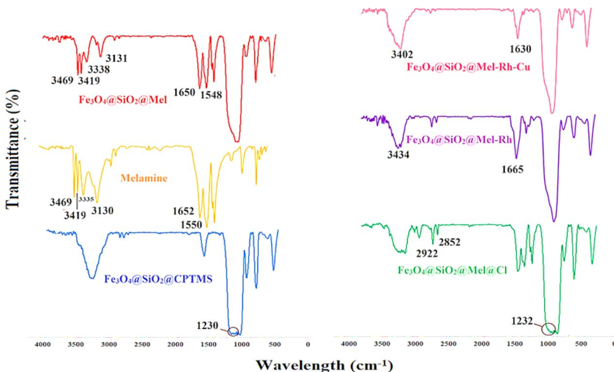
**Figure 1:** FTIR spectrum of  $\text{Fe}_3\text{O}_4@\text{SiO}_2@\text{Mel-Rh-Cu}$  synthesis steps
