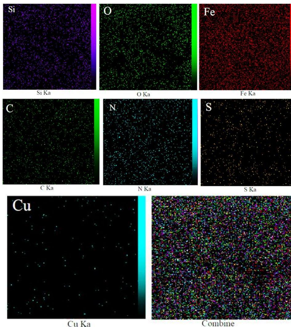
Figure 6: Elemental mapping of Fe<sub>3</sub>O<sub>4</sub>@SiO<sub>2</sub>@Mel-Rh-Cu
