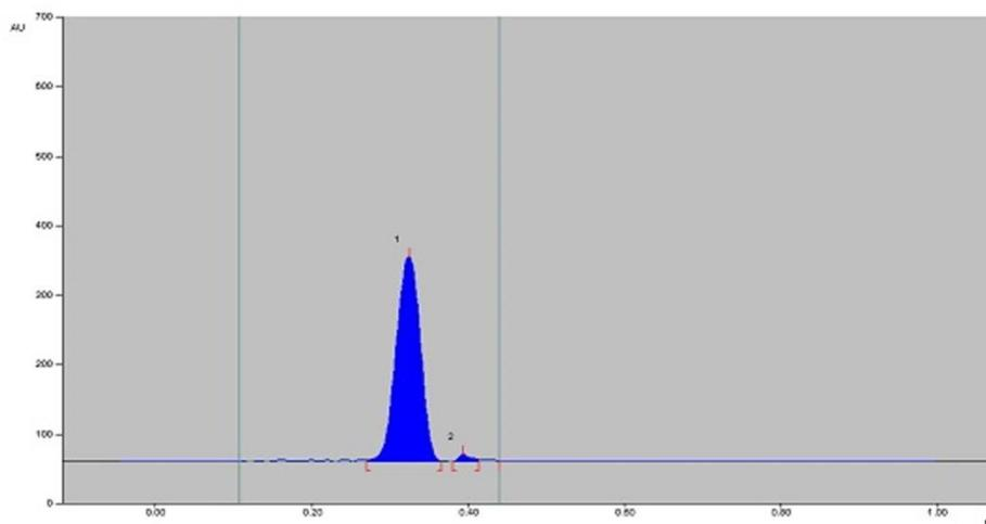
**Figure 2.** Densitogram of EDA with mobile phase *n*-hexane: ethyl acetate 7:3 (800 ng/band)
