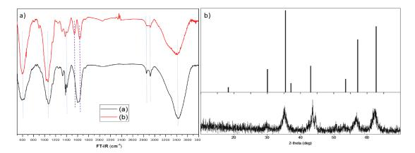
**Figure 1.** XRD pattern of SPION-chitosan and CS<sub>2</sub>-modified SPION-chitosan. FTIR spectrums of SPION-chitosan and CS<sub>2</sub>-modified SPION-chitosan
