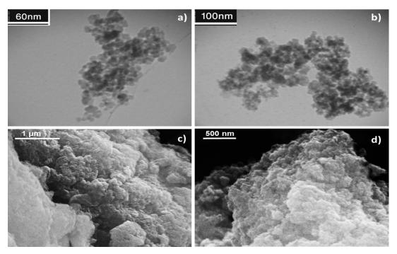
**Figure 2.** TEM images of (A) SPION-Chitosan and (B) CS<sub>2</sub>-modified SPION-chitosan. (C) SEM images of Fe<sub>3</sub>O<sub>4</sub>-chit-CS<sub>2</sub>H and (D) Fe<sub>3</sub>O<sub>4</sub>-chit-CS-lip
