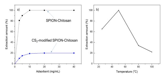
**Figure 3.** (A) Extraction of BSA in different amounts of SPION-chitosan and CS<sub>2</sub>-modified SPION-chitosan; (B) Extraction of BSA using CS<sub>2</sub>-modified SPION-chitosan at different temperatures
