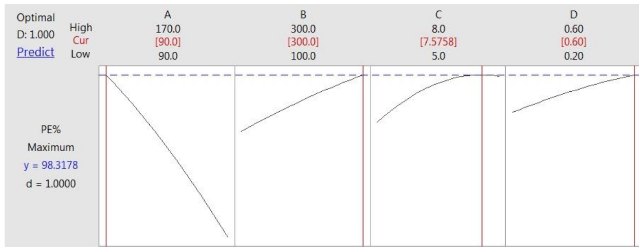
Figure S3: The optimization plot for Tra degradation efficiency with \alpha -Fe 2 O 3 nanoparticles/ 12-TSA.7H 2 O
