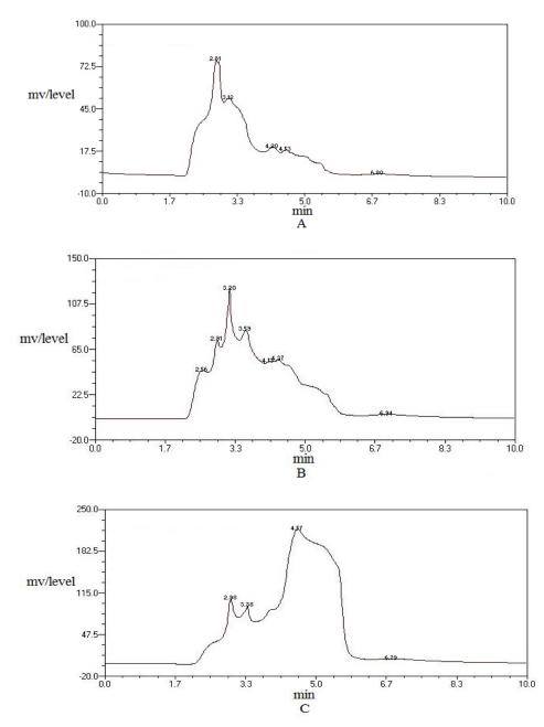
Figure 3. HPLC results by ultrasonic extraction with deionized water solvent for three different durations. A: 30 min, B: 60 min, C: 90 min
