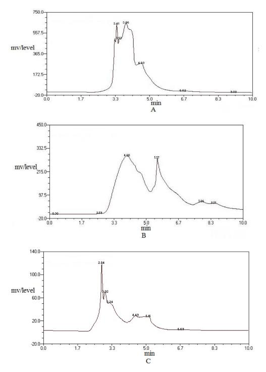
**Figure 6.** High performance liquid chromatography of extraction by soxhlet method: A: with methanol solvent, B: with chloroform solvent, C: with water solvent
