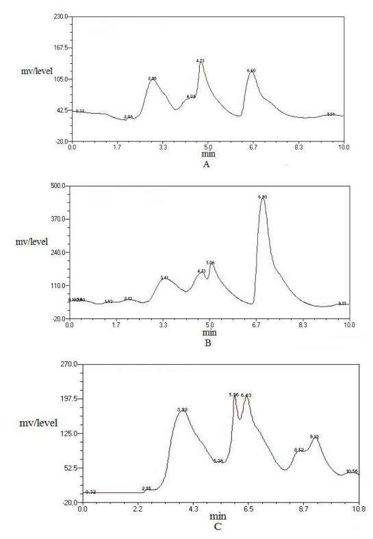
Figure 5. HPLC results by ultrasonic extraction with chloroform solvent for three different durations. A: 30 min, B: 60 min, C: 90 min
