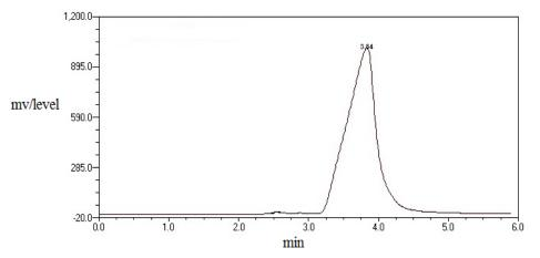
Figure 1. High performance liquid chromatography chart of the quercetin standard
