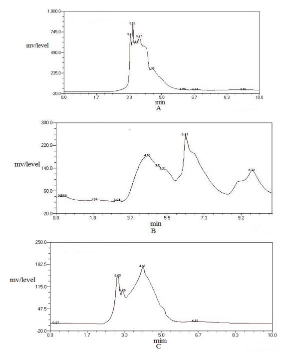
**Figure 2.** High performance liquid chromatography of extraction by soaking method: A: with methanol solvent, B: with chloroform solvent, C: with water solvent
