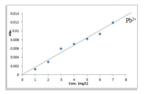
Figure 6: The calibration curve for Pb(II)
