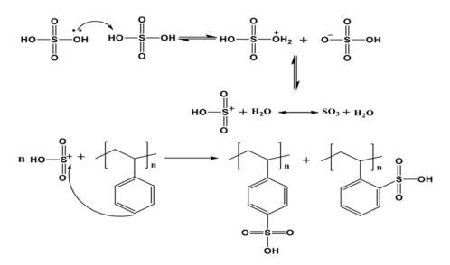
Scheme 1: Pathway of sulfonation reaction of polystyrene
