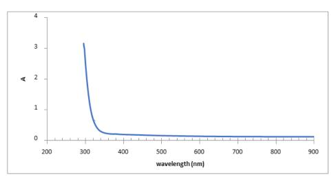
Figure 11: UV-Visible spectrum of SPS thin film
