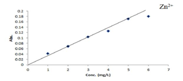
Figure 4: The calibration curve for Zn(II)
