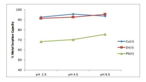
Figure 10: Percentage of metal sorption capacity by resin as a function of pH
