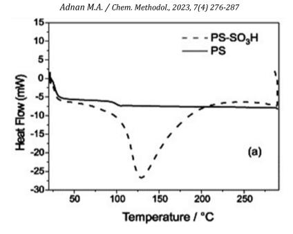
Figure 3: DSC thermogram of polystyrene and sulfonated polystyrene
