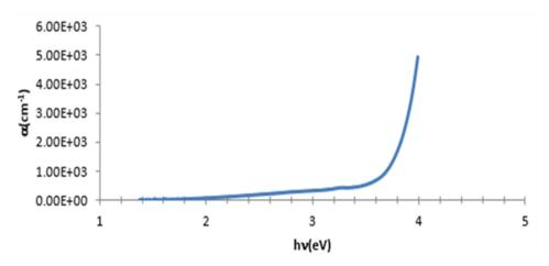
Figure 12: Absorption coefficient as a function of photon energy
