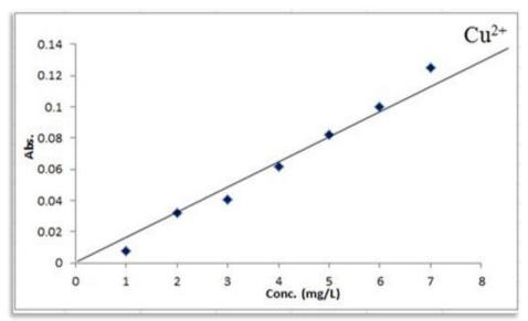
Figure 5: The calibration curve for Cu (II)
